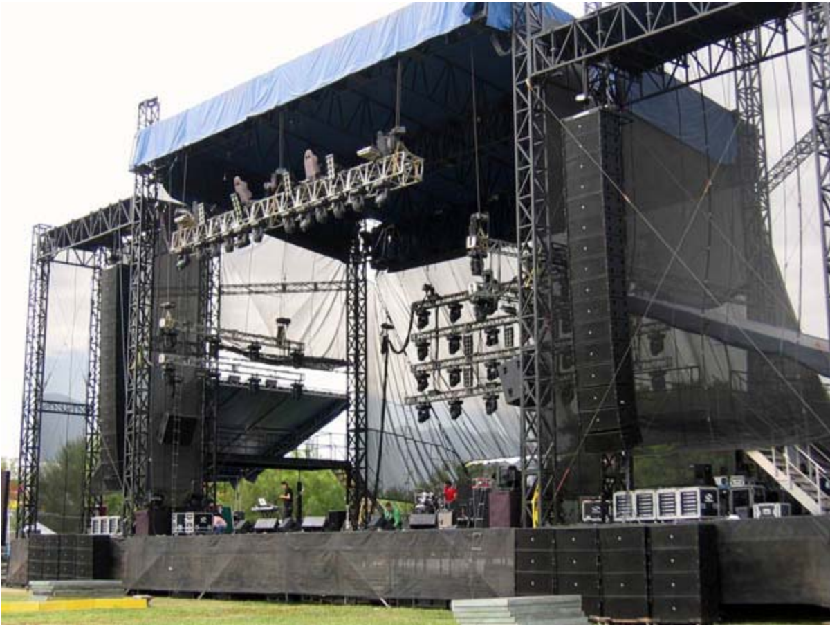
Classic “Line Array” sound system with ground level subs
